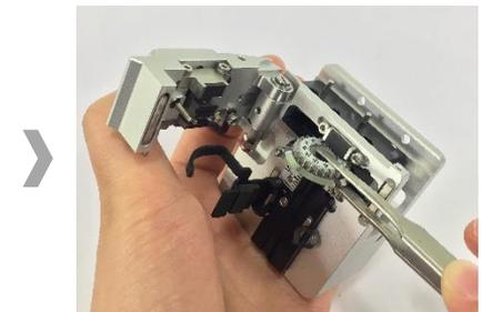
Remove old blade with blade gear from body and replace new blade with blade gear. In here reassembling should be done in a reverse order of disassembling. At this time, especially be careful not to damage the blade. Check the blade operating condition with cleaver cover.
